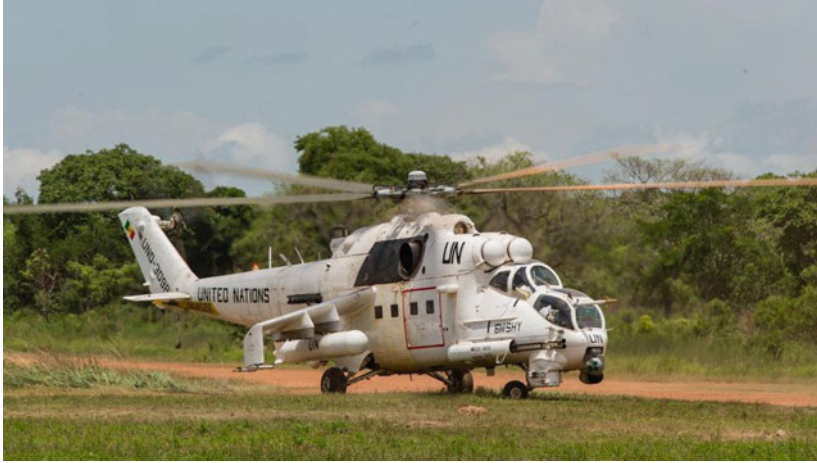
Fig. 2 The Mi-35 Attack Helicopter deployed in MINUSCA by Senegal. The camera pod is at the very front of the aircraft below the abbreviation “UN.” Also observable is a slim rocket on one stub wing alongside the larger external fuel tank. The Gatling gun is next to the gunner station, and the pilot sits higher up in the aircraft ( Source MINUSCA, 2017)
