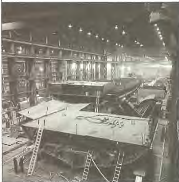
Hull sections for the first Canadian Patrol Frigate being assembled in Saint John, New Brunswick using modern modular construction techniques.
