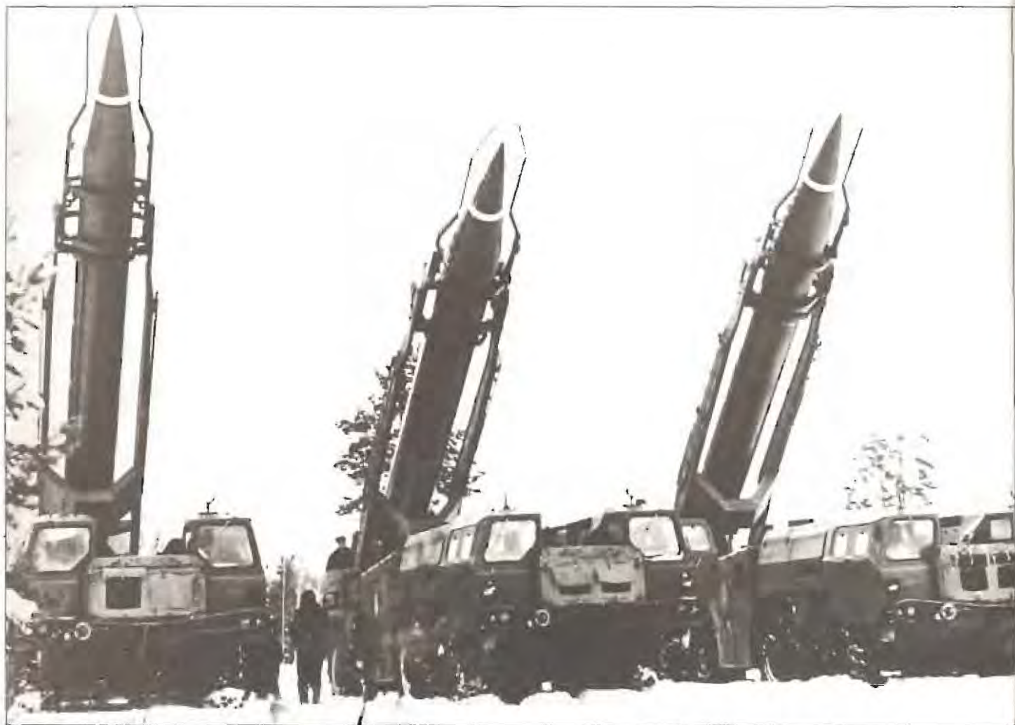
The Soviet SCUD-B surface-to-surface missile has a range of 300 km, is capable of launching nuclear, chemical or conventional warheads and is in service throughout the Warsaw Pact.
