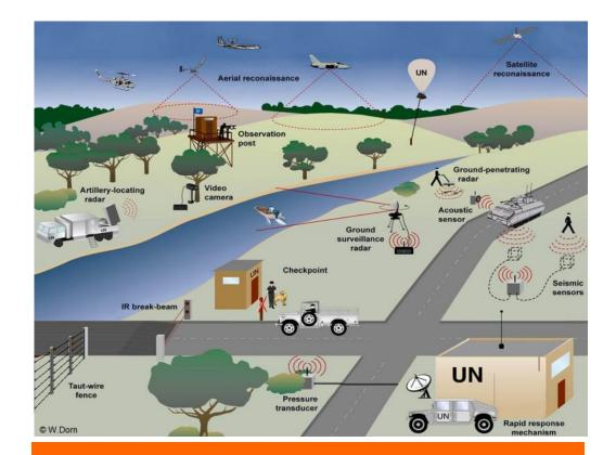
Overview of types of monitoring technologies (Source: W. Dorn, *Keeping Watch: Monitoring, Technology and Innovation in UN Peace Operations*, UN Press, 2011, —> www.keepingwatch.net)
